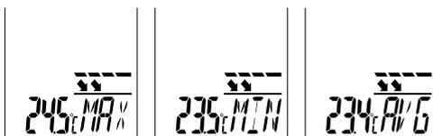
Max/Min/AVG modes refer to the infrared temperature and show the maximum, minimum or average infrared temperature. With the trigger (9) pressed, the Max/Min/AVG values are determined while measuring. The value is deleted and calculated again at the start of a new measurement or by pressing the trigger (9).
