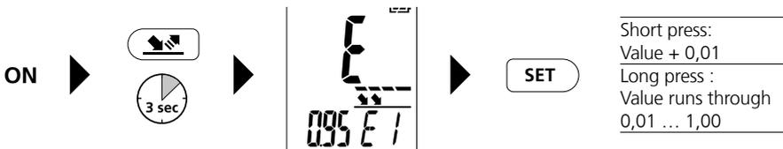
The storage locations E1 - E5 can be changed arbitrarily. By long-pressing on the storage location it can be adapted and the value remains stored. The factory reset resets the values to 0,95 / 0,85 / 0,75 / 0,65 and 0,55.
