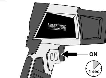
The device can also be switched on with the MODE button (4). No measurement is triggered and the last measured values are displayed.
