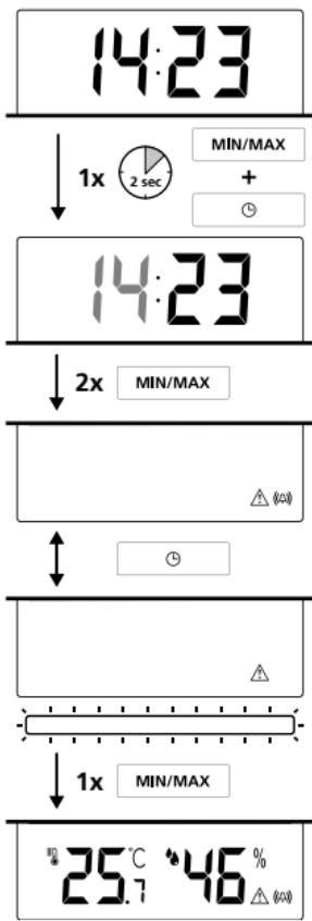
! The humidity warning can be set in the menu as an acoustic alarm, visual alarm or a combination of the two. In the event of constantly high or low humidity levels, the alarm symbol appears on the display and a visual and/or acoustic warning is generated at certain intervals. The alarm is not emitted constantly in order to save energy and avoid disturbances.
