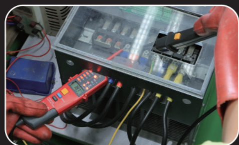
Phase rotation test
