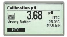
Wrong Buffer – The pH reading is not within range of the selected buffer.
