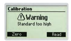
If the CAL Check™ standard value is too high, the display will show a high standard message. If this message appears, check if the correct cuvet was used.
