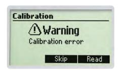
If the calculated calibration coefficients are outside a certain range a calibration error message is displayed.
