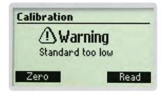
If the CAL Check standard value is too low, the display will show low standard message. If this message appears, check if the correct cuvet was used.
