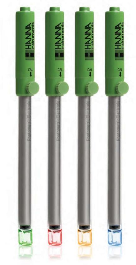
Each probe has an LED at a specific wavelength that shines light through the sample and reflected back by a platinum mirror sealed in glass. The reflective measurement has a fixed path length and allows for a high color sensitivity in a compact design.
