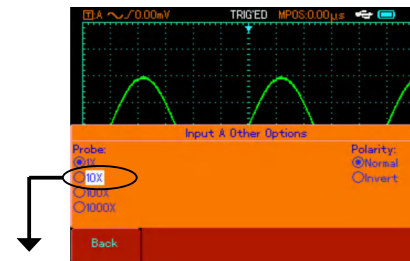
Figure 2-11 Setting the probe ratio
