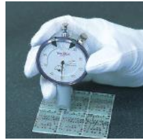
V-Grooved depth measurement of Print circuit board by using DM-251.
