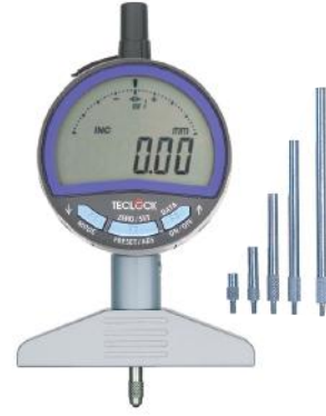
DMD-214A φ3.2 Steel Ball Contact Point ·Measuring Range 220mm ·With 5-Extension rods
