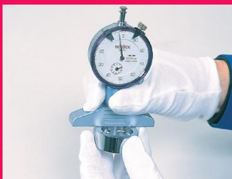
Measuring the concavity depth in work piece of which center is bored. The photo shows 2.03 mm.
