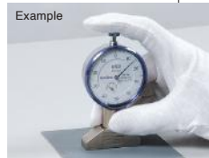
Thickness measurement of painted film waterproof stuff (measuring by pressurization)
