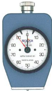
GS-750G Type B Durometer Medium-hard rubber
